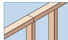
**Timbrtip** Remember that top plates must break over a stud and all top plate splices must be at least 4' from any other splice. It may be necessary to cut your top plates as you progress to ensure that they join over a stud.
